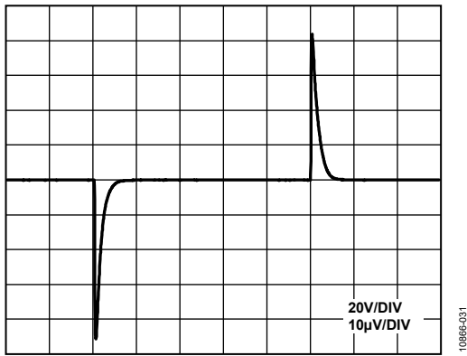
Figure 31. Operational Amplifier Load Transient Response (100 µA Load Change)
